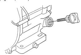
Figure 5. Engine Oil Dipstick
